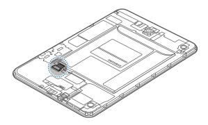
5 Peel the flap from the battery, and then pull it to remove the battery.
